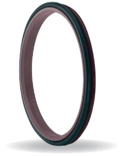
**Double Wiper PT 4**, is a two-piece wiper set, consisting of an engineered PTFE profile ring with one sealing and one wiping edge plus an O-Ring energizer.
