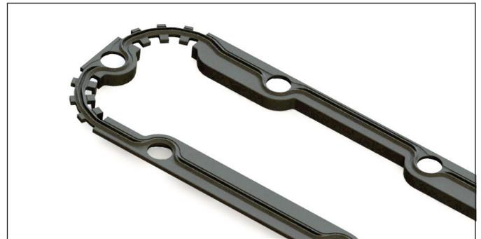
Cut-outs allow bending of straight sections to fit an oversized gasket design into the usable area of a standard mold, saving press and tooling costs.
