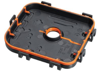
Freudenberg Sealing Technologie's 2K-Housing serves to protect electrical components from vibration and environmental damage. This innovative component integrates both the housing and a seal into a customizable lid, maximizing its protection ability. Our 2K-Housing not only serves as a static sealing solution, but it also reduces dynamic loads and optimizes the sealing function against the connecting part, providing superior tolerance compensation, even within large temperature variations.
