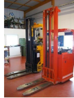
Type 2: Side loader with + w/o seat, Narrow Aisle Reach Truck
