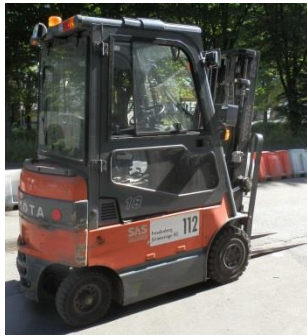
Type 1: Front loader with 3 or 4 wheels
