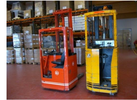
Type 2: Side loader with + w/o seat, Narrow Aisle Reach Truck
