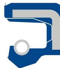
BAUM with knife-cut protective lip in NBR
