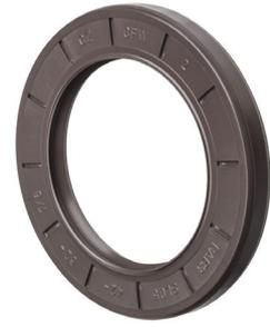
Medium pressure seals, such as the BABSL, can be used in many applications including pumps and motors in hydro-units, mechanical power transmission gearboxes, and 2-stroke engines. However in conventional seal designs, as pressure increases the seal life dramatically decreases due to atypical seal wear that is caused by pressure distortion of the seal lip geometry and increased friction at the contact point. The BABSL minimizes those problems over a wide range of operating conditions.
