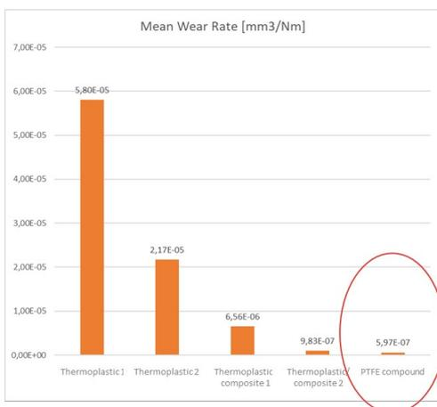
**Figure 4:** Comparison of the mean wear rate for different thermoplastics under dry friction conditions; counter surface; stainless steel Ra ~ 0,3 µm, Rz 2.5 µm
