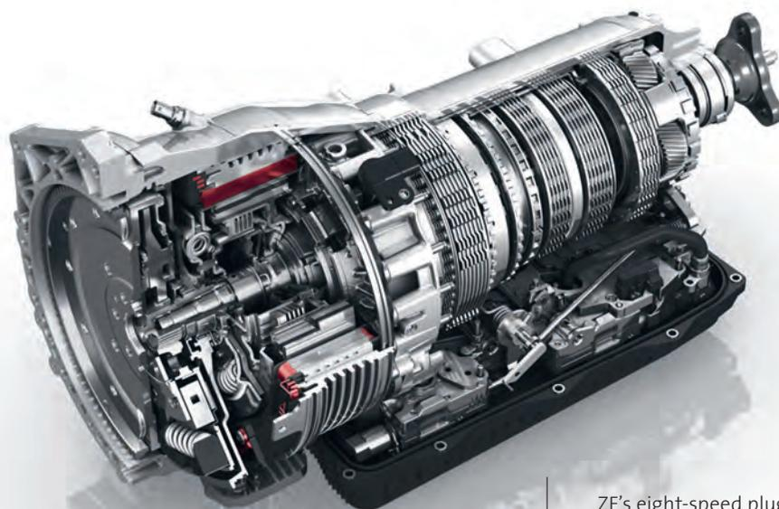
ZF's eight-speed plug-in hybrid transmission contains a powerful and compact electric motor instead of a torque converter and has the potential to reduce average fuel consumption by up to 70 percent.
