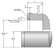
The wiper can be easily installed axially if the proper installation chamfer C is available according to the following table.
