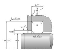
The radius R for wiper designs AE40 and AE42 is selected as follows, depending on the height of the wiper:
