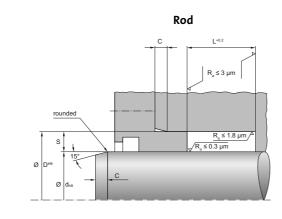
S 6 7.5-10 12.5-15 [mm] Profile width Installation slope C 3 7,5 5
