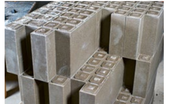
The breakthrough? Polymer resin turns ostensibly useless desert sand into polymer concrete.
