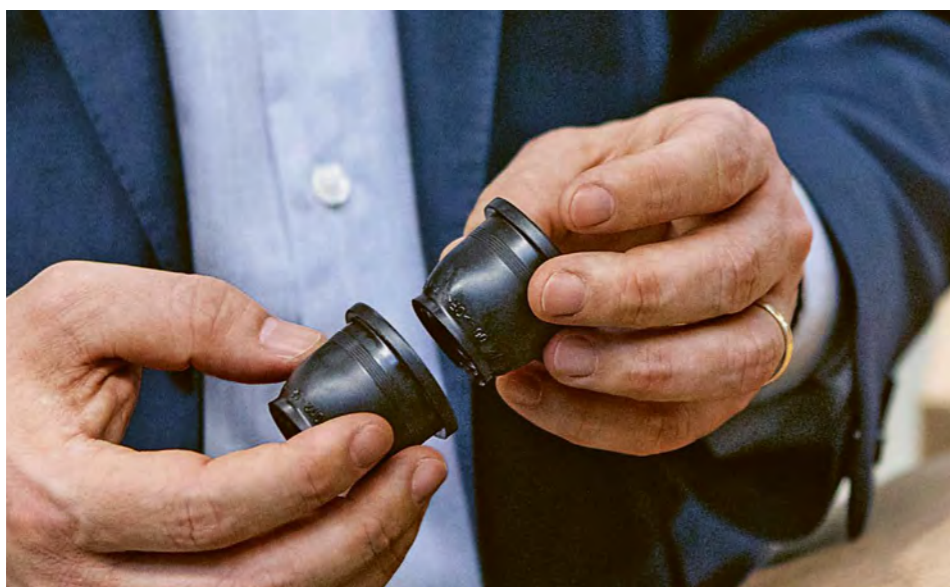
PRODUCTION Freudenberg Sealing Technologies manufactures sealing bellows and axle boots for car chassis at its Berlin-Adlershof facility.
